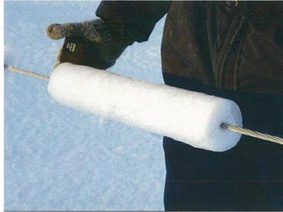
Figure 12 – Heavy radial ice buildup on a relatively small bare overhead conductor
